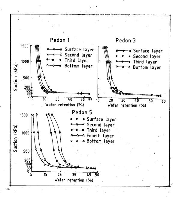
Fig. 1. Water retention at different suction in Vertisols
